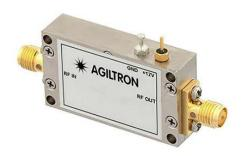
This is a high-gain, low-noise 3-stage amplifier delivering 7 Vp-p output across a broad frequency range of 30 kHz to 45 GHz. It is a general-purpose broadband driver amplifier optimized for Mach-Zehnder optical modulator applications, offering low power dissipation, high drive capability, very low added jitter, and fast rise time. The amplifier requires a 12 V DC power supply at 300 mA and features a GPPO male connector. A compatible power supply is included for user convenience.
